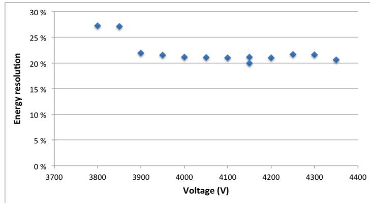
Figure 10: Energy resolution as a function of the input voltage.
