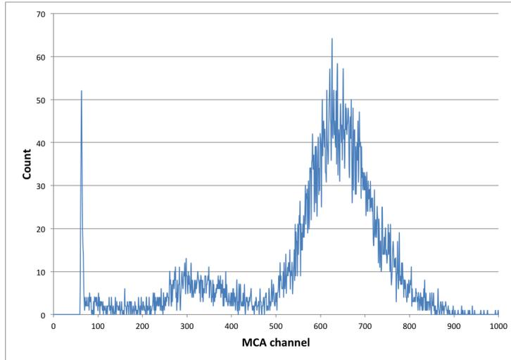
Figure 9: Triple-GEM  $^{55}\text{Fe}$  spectrum on  $\text{Ar}/\text{CO}_2$  (70/30) measured with a MCA.
