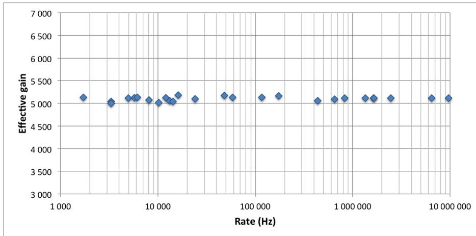
Figure 15: The gain as a function of the rate of X-rays.
