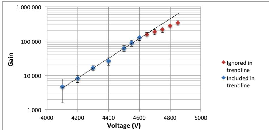
Figure 13: The gain as a function of the voltage. At high gains, there is a saturation in the graph.
