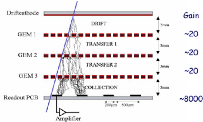
Figure 7: The avalanche process inside a triple-GEM detector.
