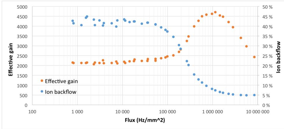
Figure 18: The ion backflow and the gain as a function of the X-ray flux.
