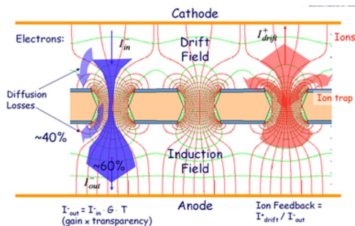
Figure 5: The principle of operation of a single-GEM detector.
