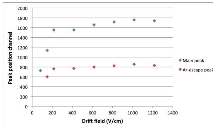
Figure 11: Peak position as a function of the drift field strength.
