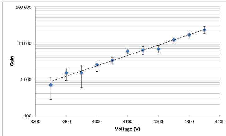
Figure 12: The gain as a function of the input voltage.
