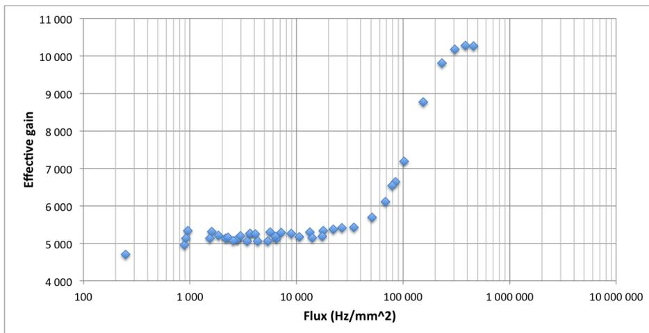
Figure 16: A graph of the gain of the detector as a function of the X-ray flux, with starting gain 5000.
