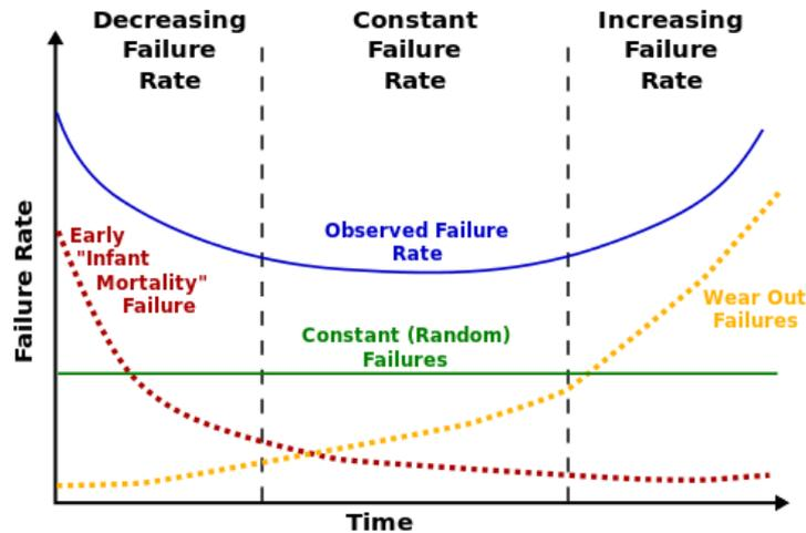
Figure 2: The figure present a bathtub curve. (The Figure is from the public domain.)
