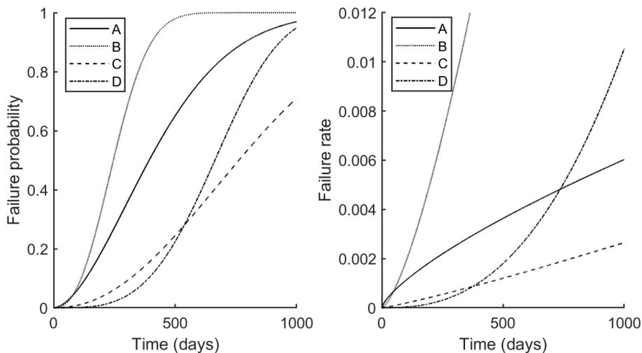
Figure 4: Failure distributions and failure rates of four different components, using Weibull distributions.
