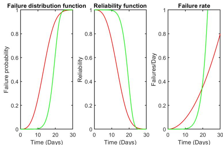
Figure 1: The figure presents failure distribution, reliability and failure rate of two different components. Both component's failure distributions are Weibull distributed.
