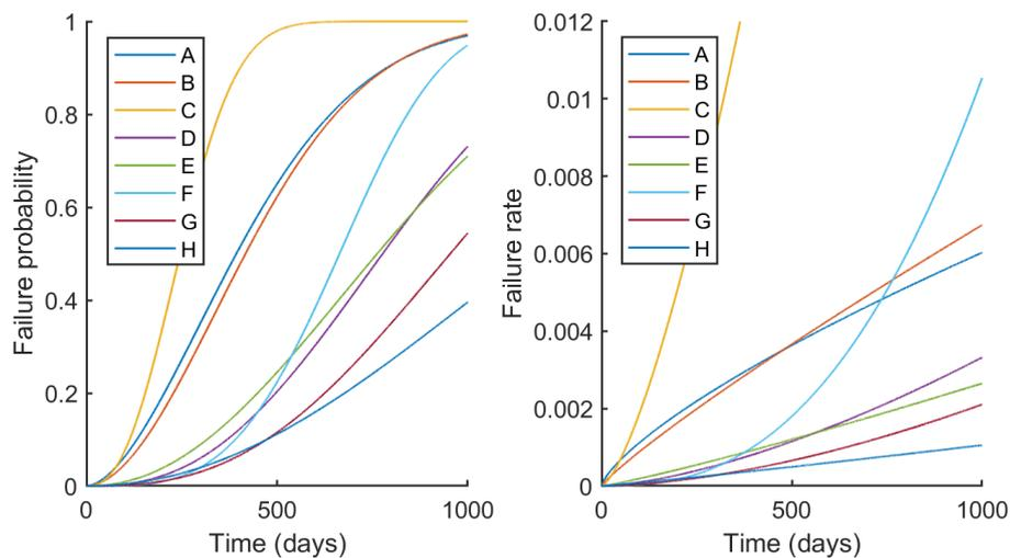
Figure 9: Figure shows failure distributions and failure rates of all components in the example system.
