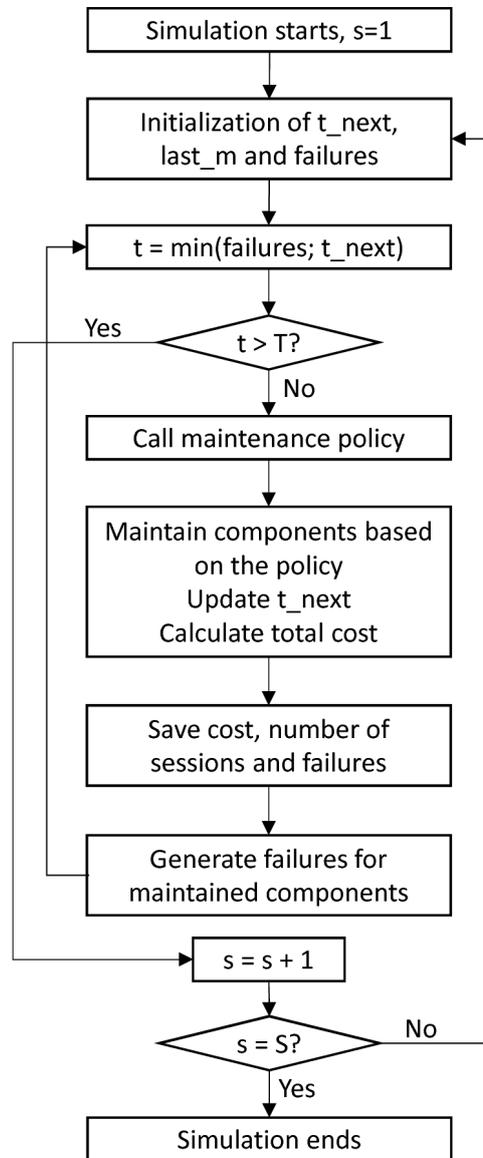
Figure 8: Chart presents how the simulation proceeds.
