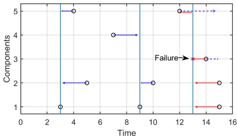
Figure 3: The individual maintenance plans are determined for each component (black dots). Then maintenance plan is made by grouping the maintenance activities (blue arrows).
