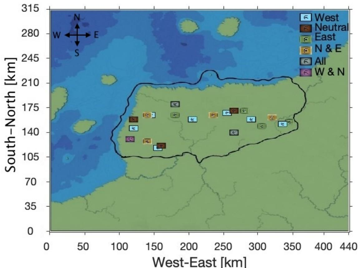
Figure 10: Radar placements of air surveillance system alternatives. The radars are depicted by colored squares. The radar's color depicts which system or systems it belongs to.
