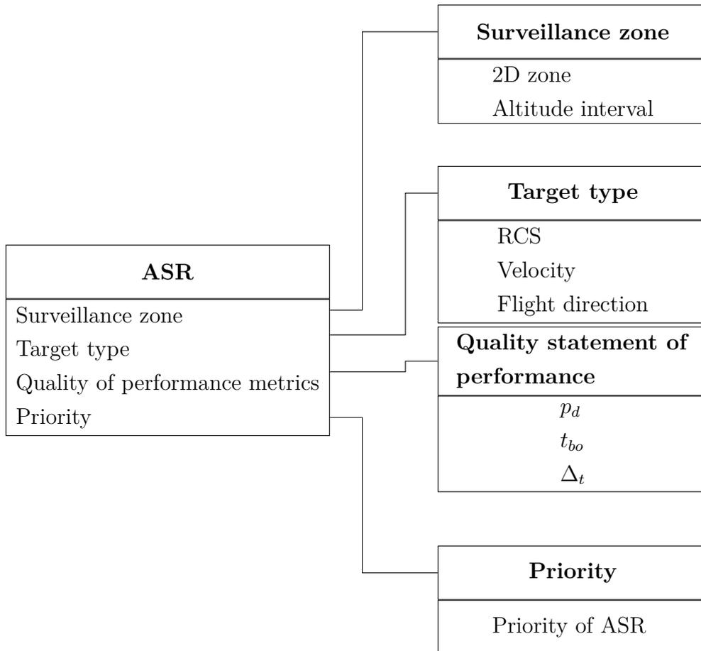
Figure 3: Definition of air surveillance requirement. The abbreviations  $p_d$ ,  $t_{bo}$  and  $\Delta_t$  stand for the probability of detection, time between observations and accuracy of track, respectively.
