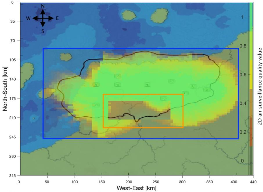
Figure 8: Visualization of the 2D air surveillance quality value taking into account multiple ASRs simultaneously.
