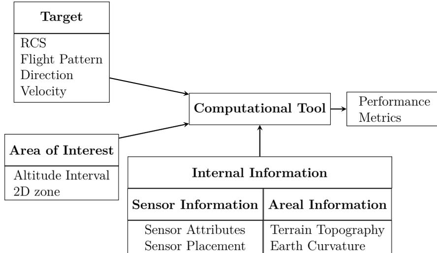
Figure 1: Inputs and outputs of the computational tool.
