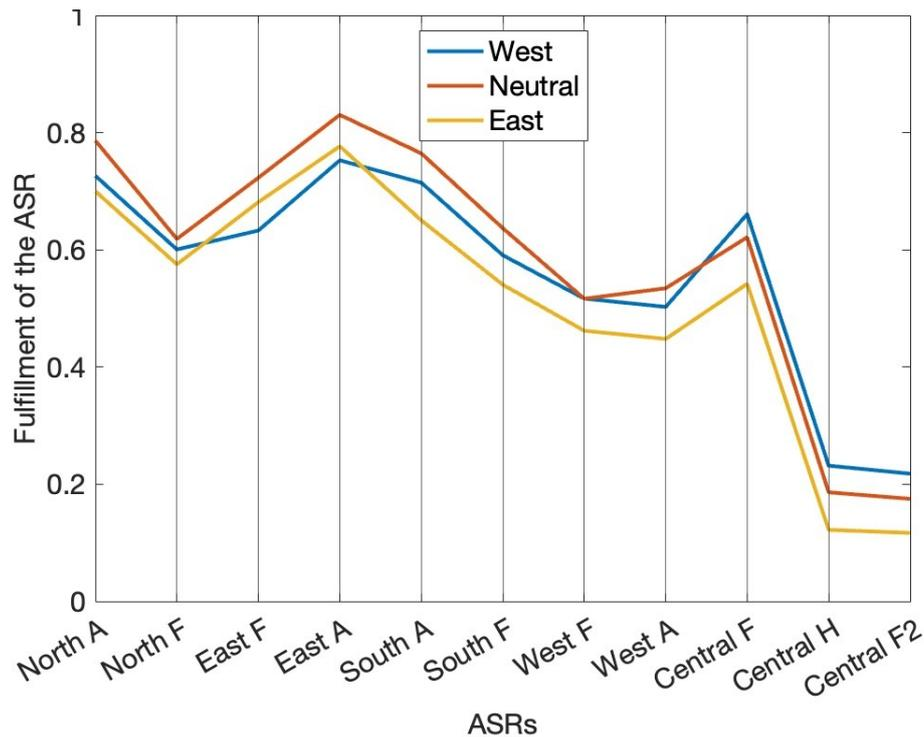
Figure 23: Fulfillment of the ASRs for the air surveillance systems. The abbreviations 'F', 'A', and 'H' stand for 'Fighter jet', 'Airliner', and 'Helicopter', respectively.
