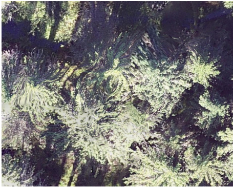
(a) Stretching issues in 2020 orthomosaic
