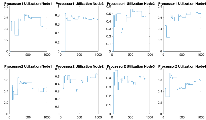
(a) Subfigure 7a: The first 1000 simulation seconds illustrate 16 active tasks populating the nodes in the beginning of the simulation run. Utilization varies between 80% to 40% in the nodes.
