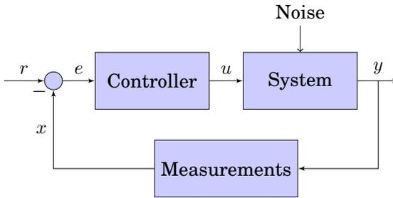
**Figure 2.1.** A simple conceptualization of a state-feedback control system.
