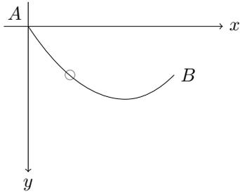
**Figure 1.1.** What kind of a curve would minimize the time for a bead to reach point B from point A?
