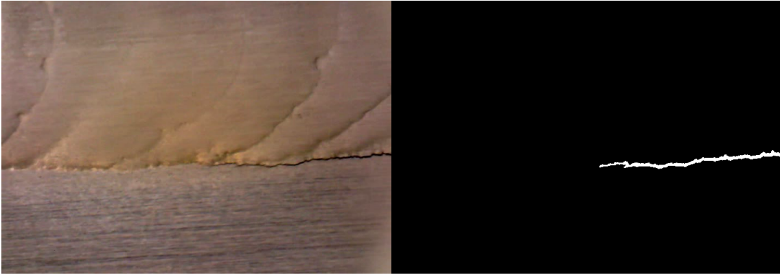
Figure 2: Example laboratory flaw with the original SD image on the left and hand annotation on right. The image represents a typical flaw which might occur at weld borders.
