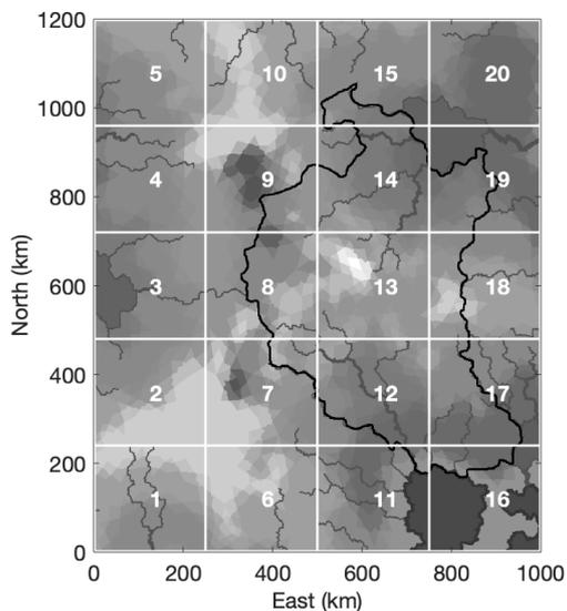
Figure A15: Radar positioning: regular division into 20 subregions.
