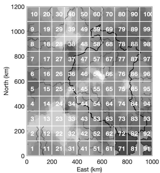
Figure A19: Radar positioning: regular division into 100 subregions.
