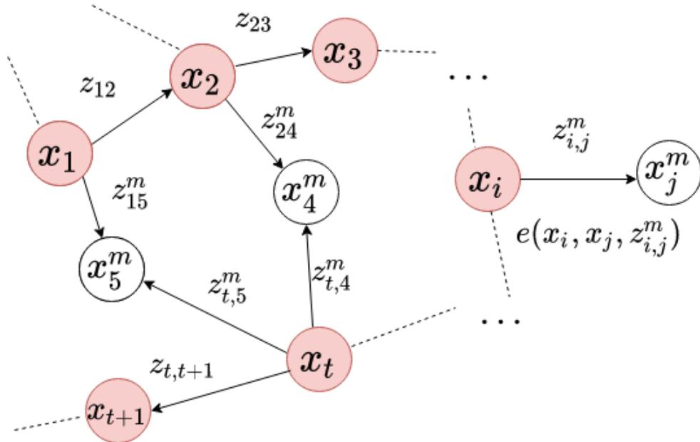
Figure 4: An example of an optimizable graph that is used for creating the objective function. For clarity, the tree observations are labeled white and marked with upper index  $m$  while scanner poses are labeled red. Note that edges between tree observations and scanner poses take into account only location data while the edges between consecutive poses use both location and orientation data.
