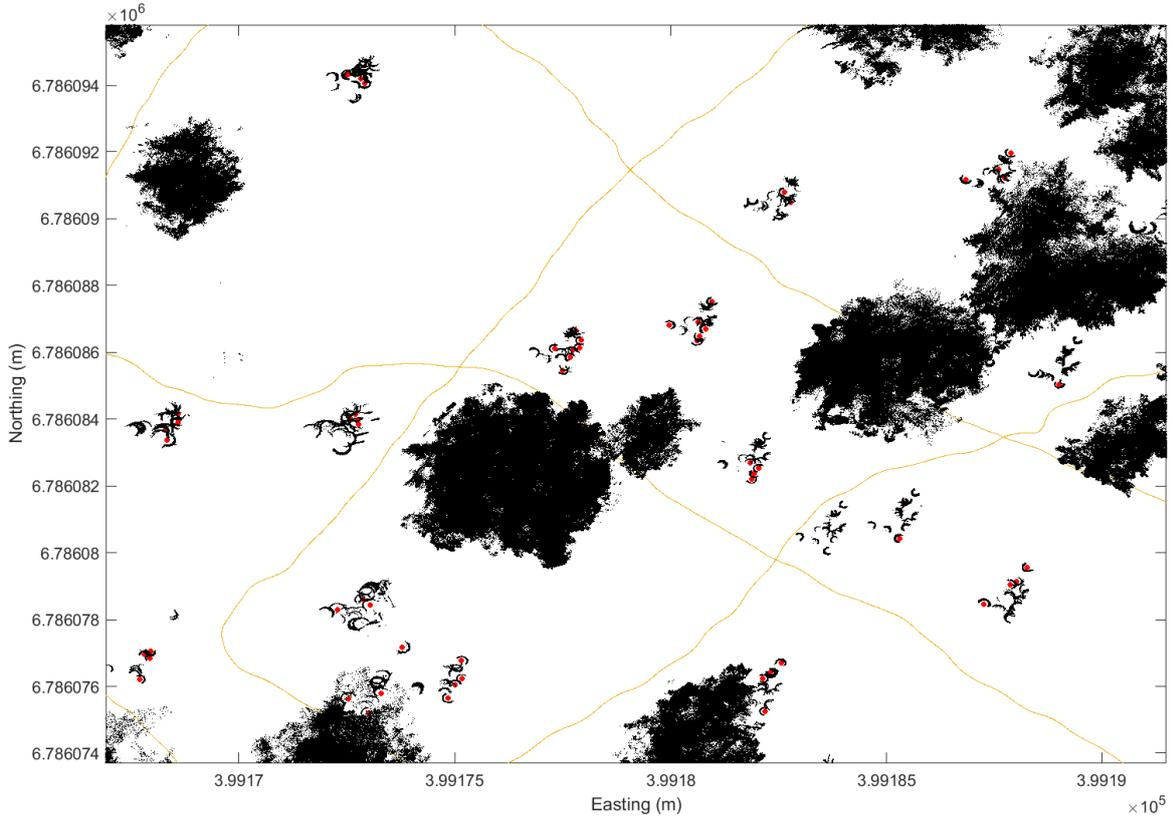
Figure 3: Example of tree detection in Plot 1 point cloud environment (top view) Black represents points in the point cloud with a z-coordinate between 3-3.5 meters. Red represents detected tree trunks from the point cloud with arc detection and orange line represents laser scanner trajectory. The multiple clustered arc-like figures can be considered to be errors in point cloud due to GPS-deterioration and the respective arc detections are assumed to be from the same tree.
