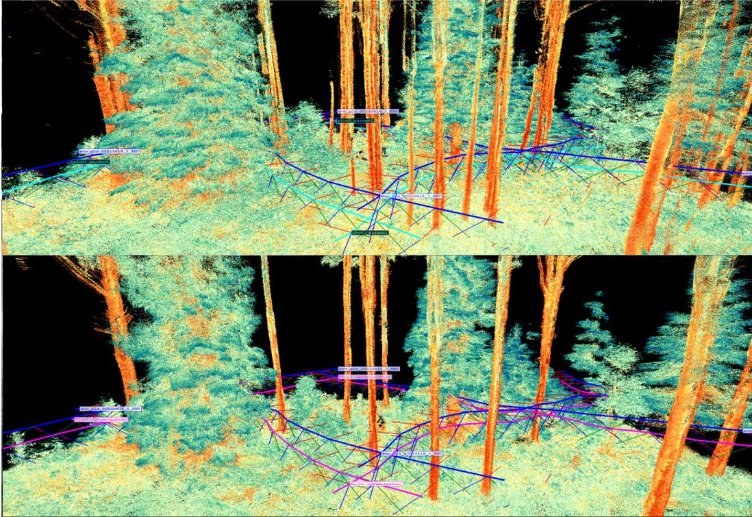
Figure 7: Example of accuracy improvement in part of Plot 1 point cloud visualization. The upper picture represents the unoptimized point cloud and the bottom picture represents the optimized point cloud. Dark blue plot represents the unoptimized trajectory. Pink and turquoise both represent the same optimized trajectory. This figure was produced by Antero Kukko
