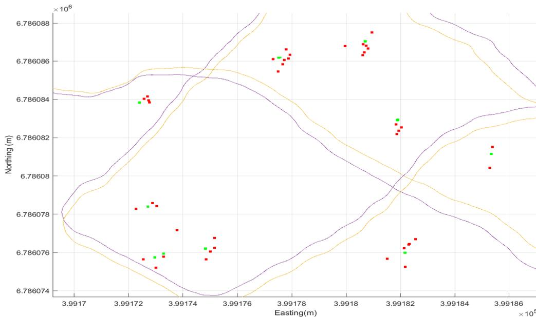
Figure 5: Visualization of some of the decision variables  $\mathbf{x}$  prior and after the optimization in forest sample Plot 1. Yellow line shows the initial trajectory and red points show the initial observations. Purple line shows the optimized trajectory and green points show the optimized observations.
