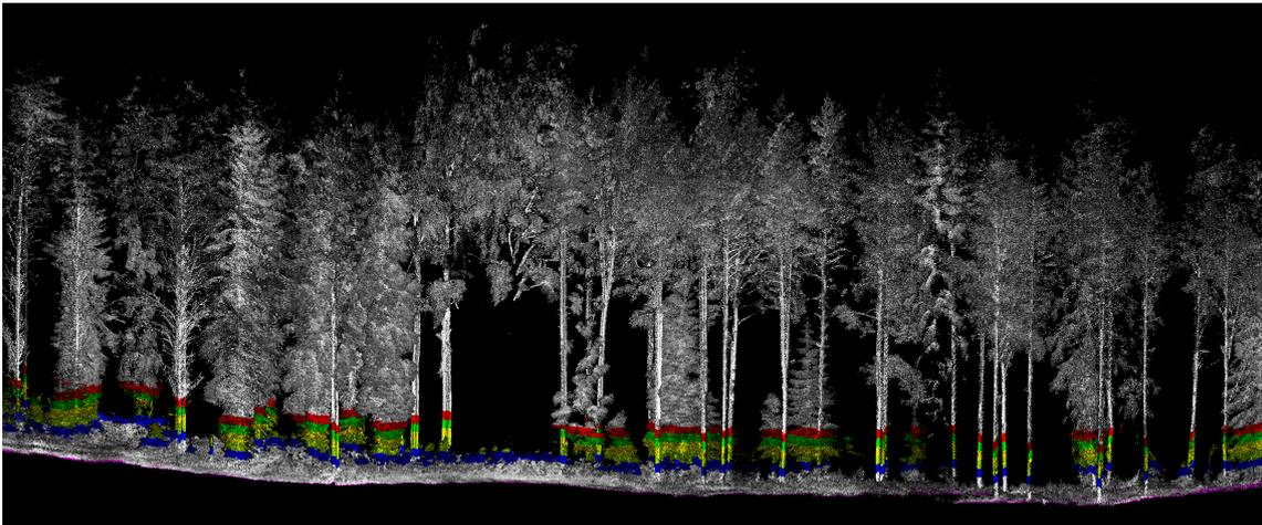
Figure 1: An example of a 3D map cross section of a forest in a point cloud format. The colored bars near the ground are colored height intervals of the point cloud. The empty area in the middle of the picture is the blind spot of the laser scanner, which can be interpreted as part of the scanner trajectory. The picture was processed by Antero Kukko.
