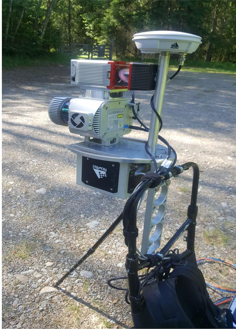
Figure 2: The backpack mounted laser scanner and GNSS/IMU -equipment for simultaneous trajectory data and point cloud data collection. The picture was taken by Antero Kukko.
