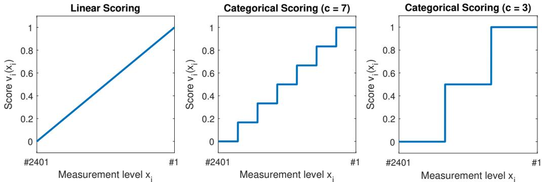
Figure 6: Three shapes of the single attribute value function.  $c$  denotes the number of categories in categorical scoring. The measurement levels  $x_i$  are ordinal rankings, where #1 denotes the best and #2401 the worst COA with respect to attribute  $i$ .
