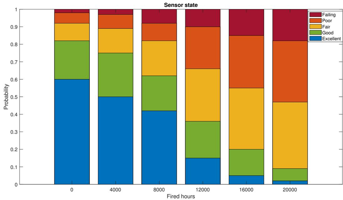
Figure 3: Probability distribution for *Sensor state*.
