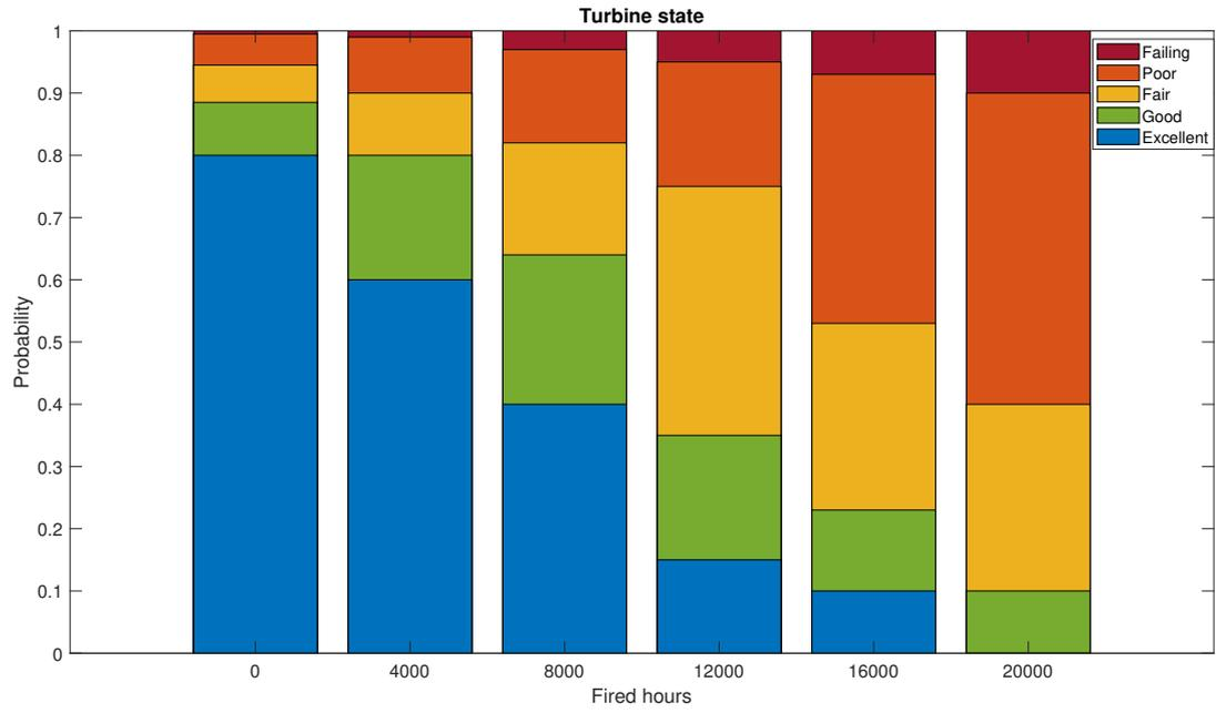
Figure 2: Probability distribution for *Turbine state*.
