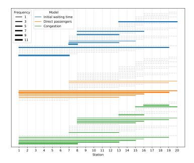
**Figure 16:** Line concepts  $(\mathcal{L}, f)$  obtained with the three models. Models solved in the passengers' perspective on the 20-station PTN with unicentric demand profile and the original terminals  $\{1, 7, 8, 13, 15, 16, 19, 20\}$ . Fleet size is constrained to 28 trains.
