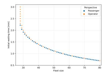
**Figure 6:** Outline of the Pareto frontier given by the solutions of initial waiting time model in both perspectives, using the  $\varepsilon$ -constraint method with varying bounds. The unicentric demand profile on the 20-station PTN is used.
