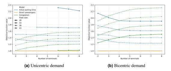
**Figure 9:** Objective function values of the three models versus the constraint for the number of terminals. Passengers' perspective models solved on the 20-station PTN with both demand profiles and four fleet size constraints. The objective function values of the direct passengers and the initial waiting time models are divided by the total number of passengers, resulting in the ratio of direct passengers and the average initial waiting time for a single passenger, respectively.
