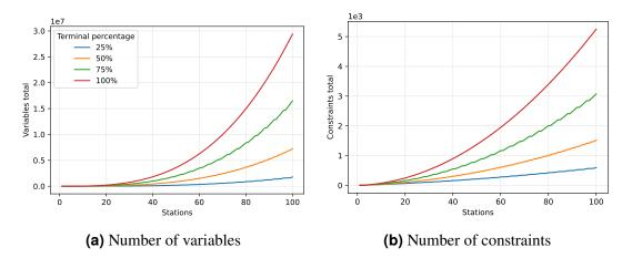
**Figure 3:** Number of variables and constraints in the initial waiting time model with a variable size linear PTN. The line pool consists of all possible lines. The terminal percentage indicates how many stations act as terminals. Terminal constraints are not applied.  $f_{\text{max}} = 60$ .
