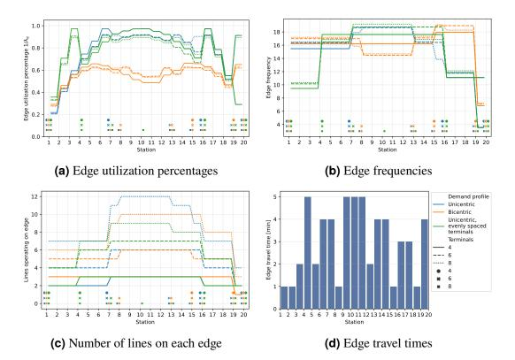
**Figure 12:** Terminals' effects on edge utilization, edge frequencies, and number of lines on edges. The congestion model solved in the passengers' perspective on the 20-station PTN with both demand profiles. Fleet size is constrained to 30 trains. The included terminals are visualized as markers on the bottom of the figures, on the corresponding stations.
