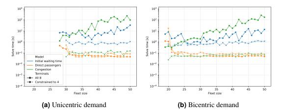
**Figure 8:** Solving times of the models versus the fleet size constraint  $\mathcal{F}$ . Passengers' perspective model solved with and without the terminal constraints on the 20-station PTN.
