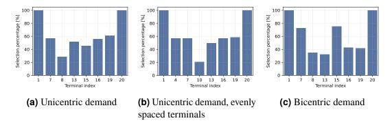
**Figure 11:** Percentage of runs for which the terminals are included in the line concept. Results aggregated from Figure 10. The initial waiting time model solved in the operator's perspective on the 20-station PTN with both demand profiles.
