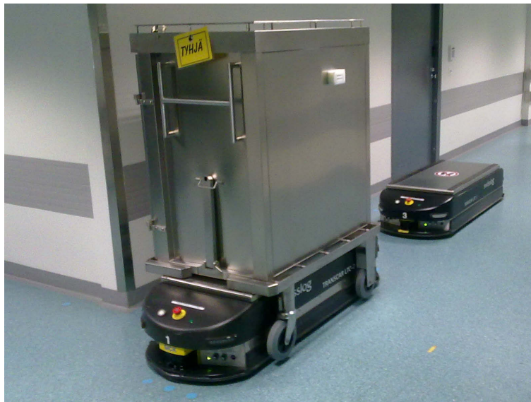
Figure 3.1: An automated guided vehicle transporting a cart and another vehicle traveling empty at Päijänne Tavastia Central Hospital in 2010. The image is cropped from the original picture taken by Petri Niemi (2010). Copyright permission is granted by EP-Logistics Ltd.
