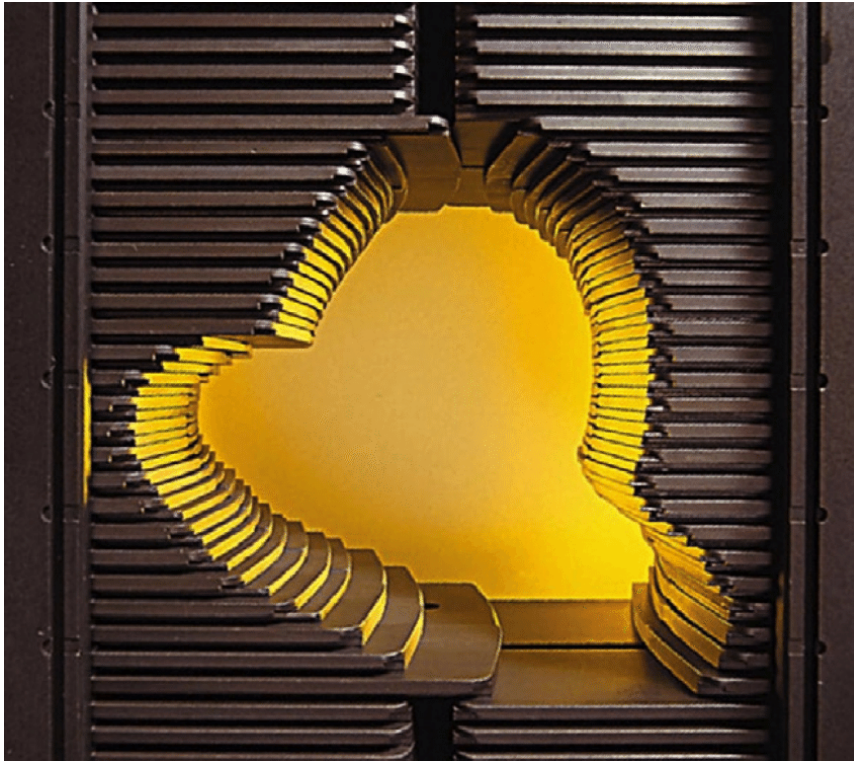
Figure 1: A multileaf collimator consists of radiation absorbing tungsten leaves, which can be moved individually allowing complex beam shapes. Picture from Varian Medical Systems, Palo Alto, California. [Source: Bortfeld [4]]
