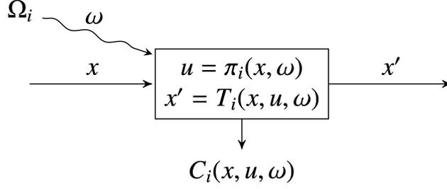
**Figure 9:** A diagram representing how the controls, incoming state and outgoing state are connected by the transition function. Source [39].
