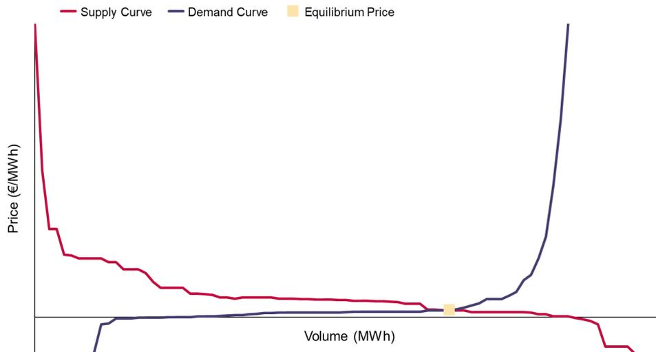
**Figure 4:** The supply (red curve) and the demand (blue curve) are represented in a Volume - Price coordinate system. The equilibrium price is located at the intersection of the supply and demand curves.
