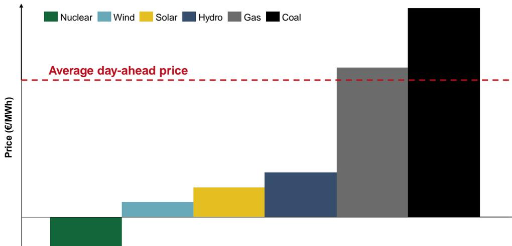
**Figure 3:** A hypothetical merit order in a bidding zone with nuclear, wind, solar, hydro, gas and coal-powered generation.
