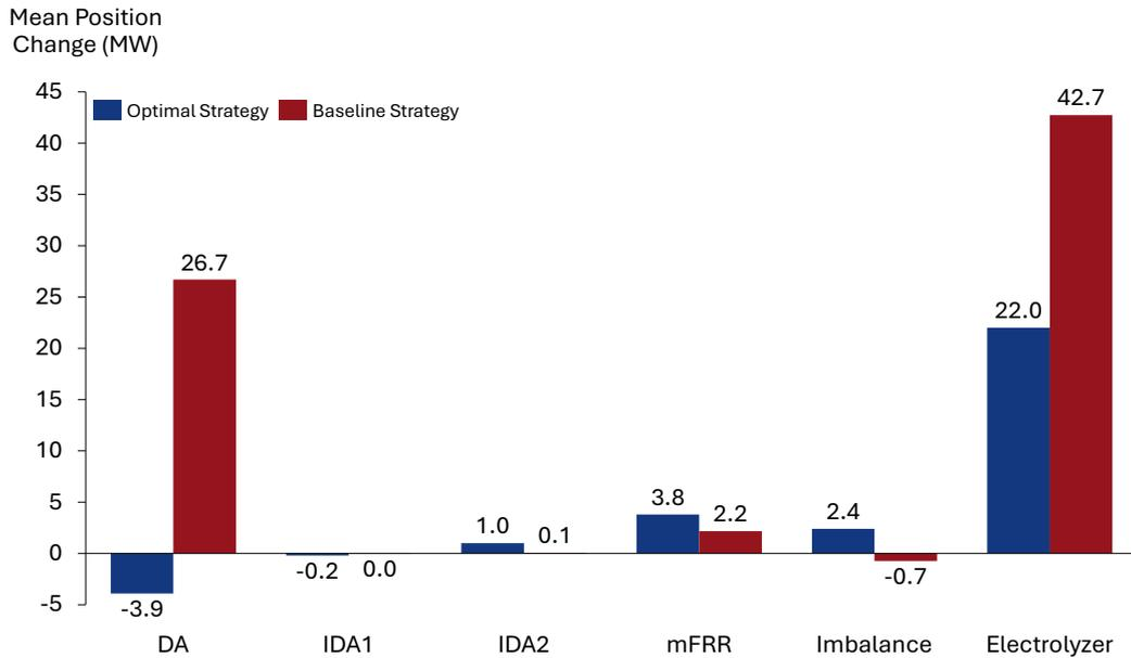
**Figure 22:** The average change in position, i.e., average sale, generation or purchase, for each profit generating source. The electrolyser contains both RFNBO and Non-RFNBO hydrogen.
