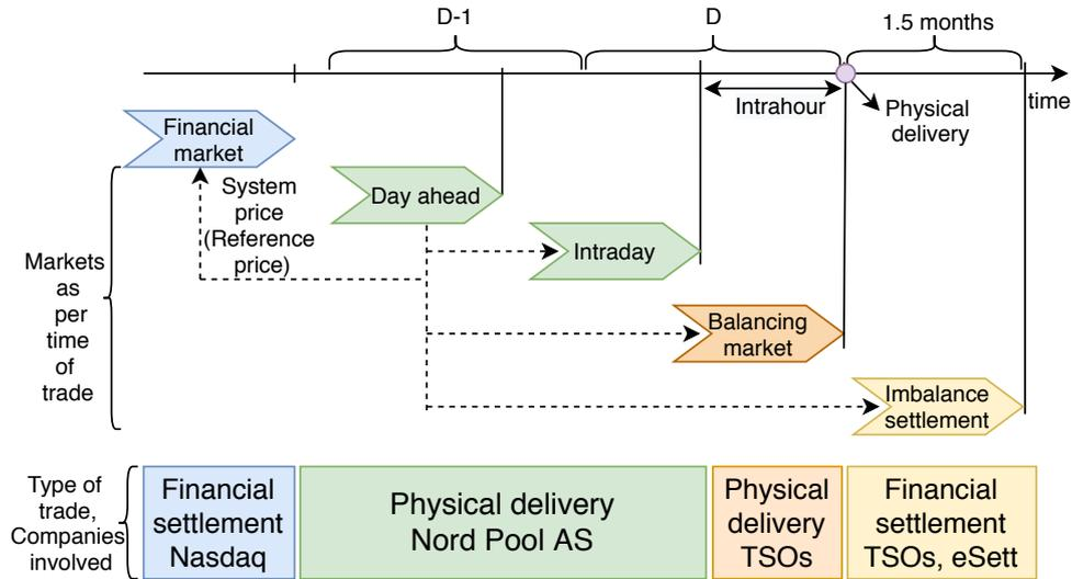
**Figure 1:** The chronological timeline for trading electricity for a single delivery hour. The figure is from [8].
