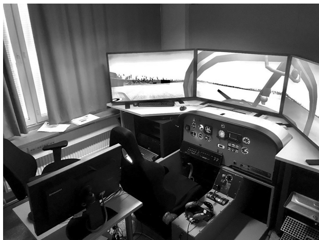
Figure 1. Vinka flight training device. The instructor's operation station is behind the pilot's seat.
