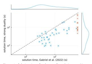
Figure 1. Solution times for the two formulations on 50 random instances with 2 producers, 5 energy sources, 3 nodes, and 3 representative days. If one of the methods failed to find a solution within 3600 s, an orange marker is used, and the marginal distributions on the right and top sides exclude unsolved instances.
