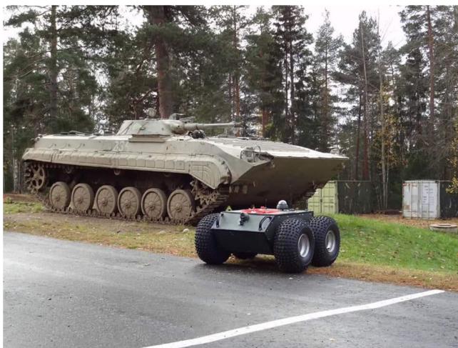
FIGURE 1 | Laykka X.3 with a loitering mine module and an armored infantry fighting vehicle in the background. [Color figure can be viewed at wileyonlinelibrary.com ]
