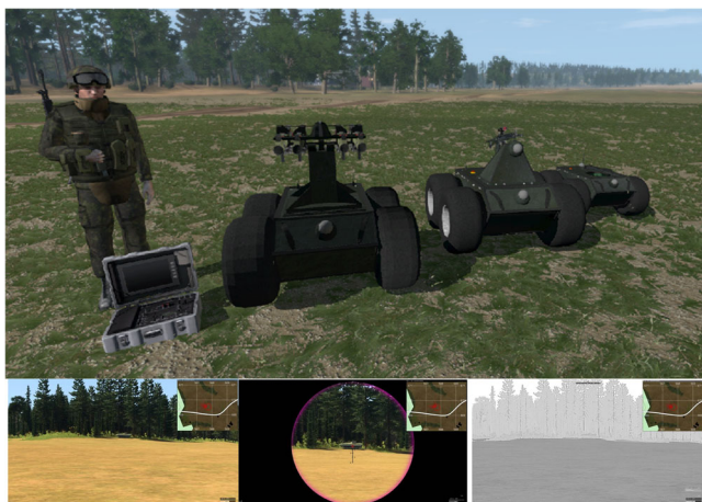
FIGURE 4 | Top picture represents the VBS visualization of the Laykka models including anti-tank, reconnaissance and loitering mine modules positioned from left to right. In the leftmost side picture, a command terminal is situated on the ground in front of an UGV operator. Three views from Laykka's cameras are in the bottom picture. The leftmost picture displays the view from the front camera, middle one from the reconnaissance module's rifle scope camera and right one from the thermal camera. [Color figure can be viewed at wileyonlinelibrary.com ]
