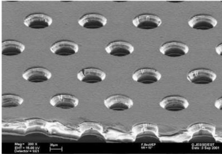
Figure 3: Image of a standard GEM foil, taken with an electron microscope. [14]
