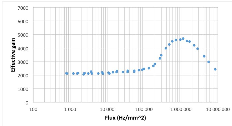
Figure 17: Another measurement of the gain as a function of the X-ray flux, with starting gain 2000.
