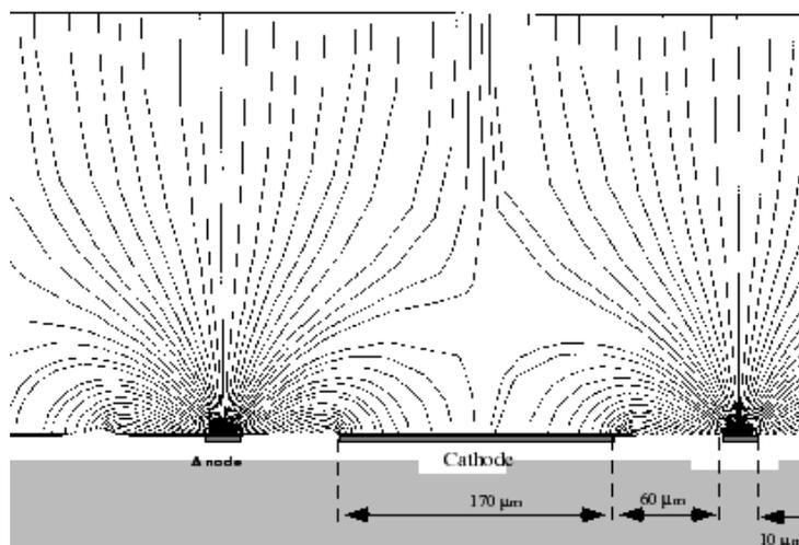
Figure 2: The structure of a microstrip gas chamber.
