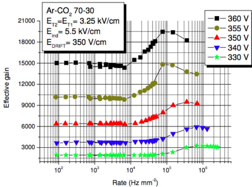
Figure 4: The gain of the detector as a function of the flux. The different colors represent different values of voltage applied to the GEMs. [19]
