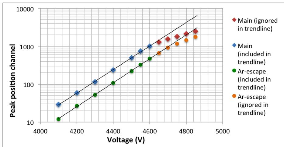
Figure 14: The saturation is also observable in the graph of the peak positions as a function of the voltage.
