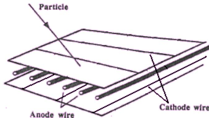
Figure 1: The principle of operation of a multiwire proportional chamber. [10]
