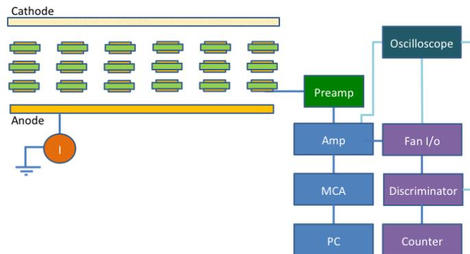
Figure 8: The setup of the measurements with the triple-GEM detector.
