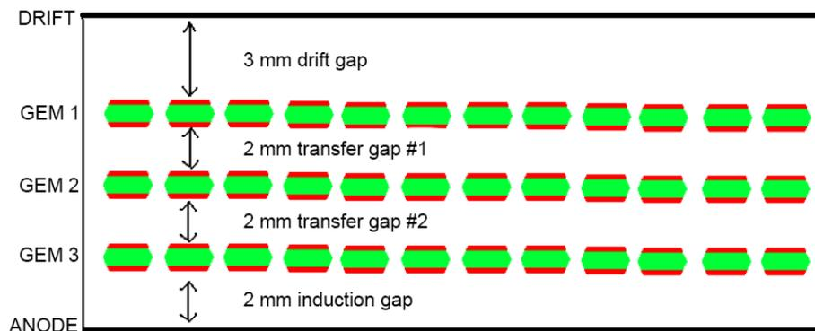
Figure 6: The structure of a triple-GEM detector. Based on the figure by Everaerts [19].
