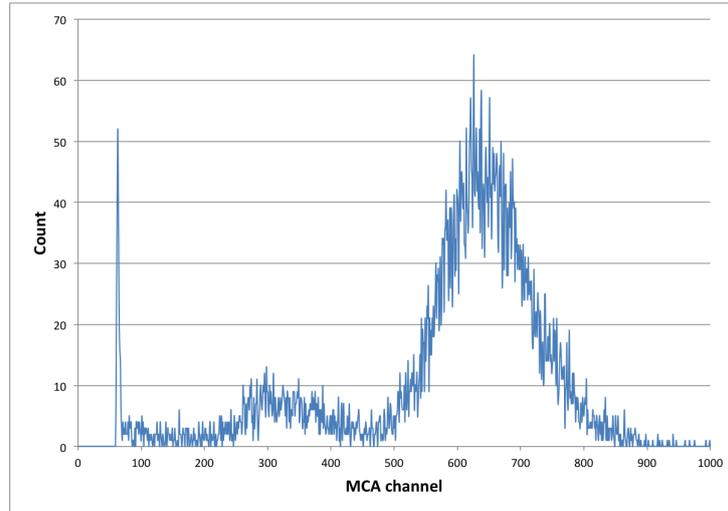
Figure 9: Triple-GEM  $^{55}\text{Fe}$  spectrum on Ar/CO<sub>2</sub> (70/30) measured with a MCA.
