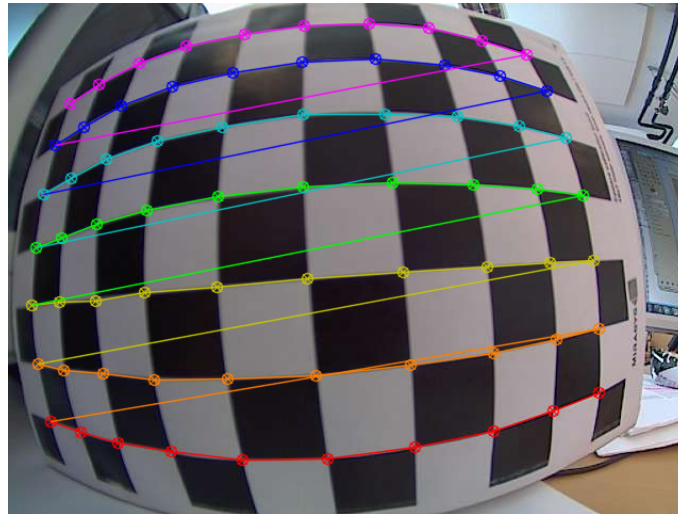
Figure 3: Heavily distorted image of a checkerboard calibration board. The image is distorted by the fish-eye lens in the camera. Detected checkerboard pattern is visualized with colored lines.
