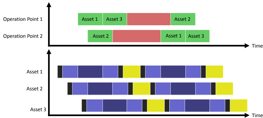
Figure 3.3. Example of a schedule. The operation area has been reduced into two operation points. The colors are the same as in Figure 3.1, except that the take off and landing delays have been embedded into the cruise flight. At the operation points green marks an asset present and pale red marks a deficit.
