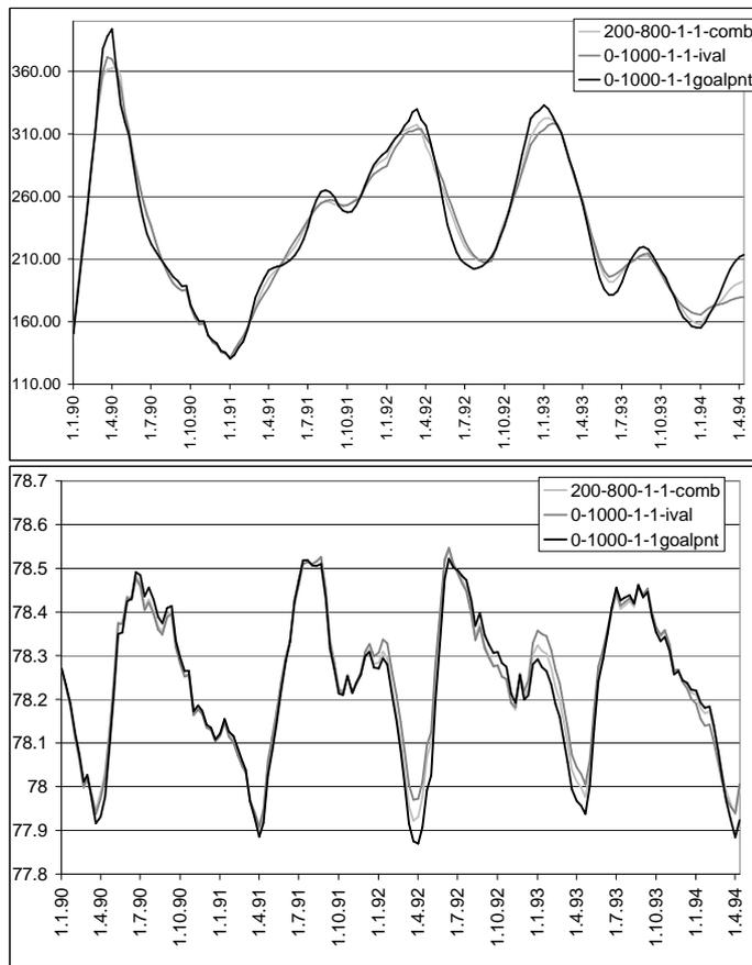
Figure 4: Regulation results for 1990-1994 outflows and water levels for different strategies with a high outflow rigidity parameter
