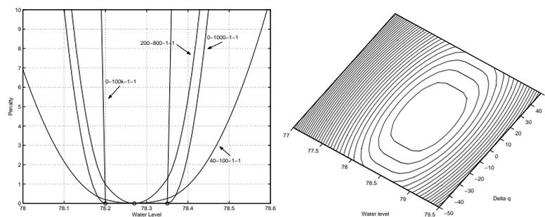
Figure 3: The penalty function (left) with different parameters and a contour plot (right) with  $c_g=40, c_i=1000, c_r=1$
